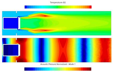
Segment of a MicroMix gas turbine combustion chamber
